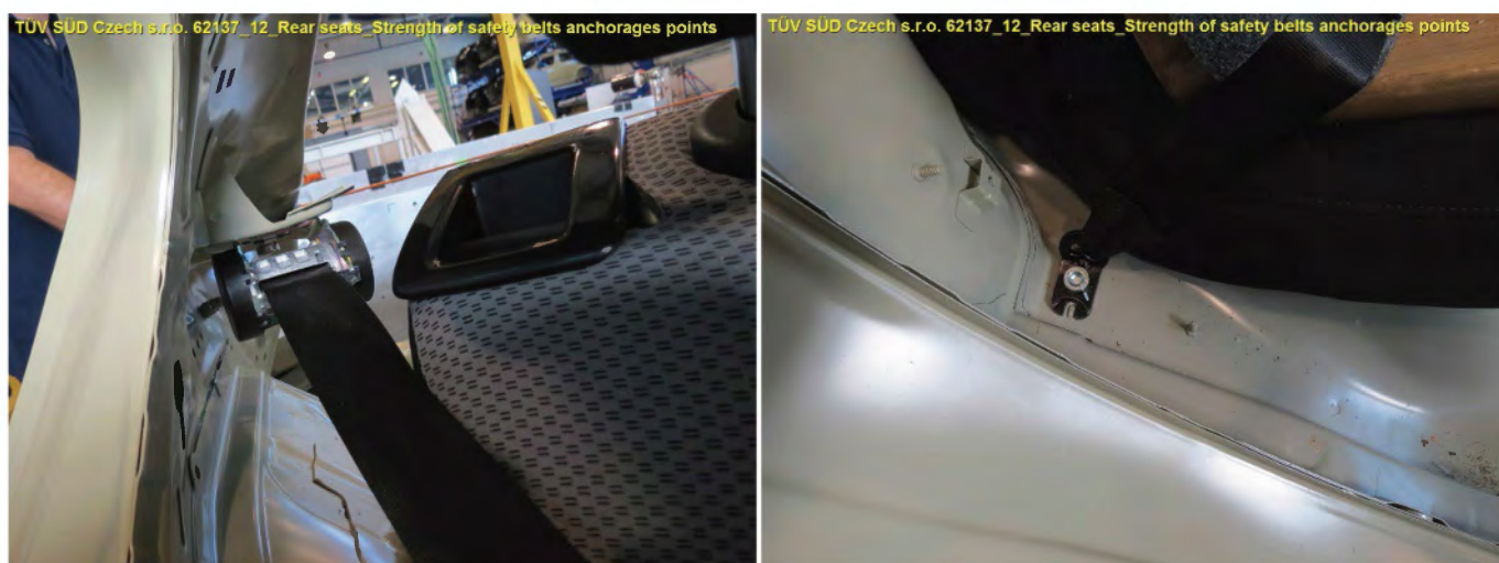
Obr. 11 a 12 Stav úchytů zadní sedačky po zkoušce. Fig. 11 and 12 Condition of the rear seat attachments after the test.
